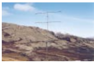
Three-Frequency Riometer Peter Stauning, Danish Meteorological Institute
